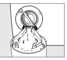
Place a suitable container under the access flap.
